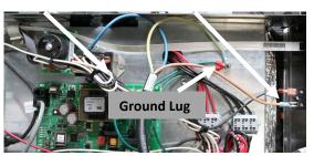
**Step 10:** Route cord leads to relay, circuit breaker, ground lug: blue to relay; brown to circuit breaker; green/yellow to ground lug.
