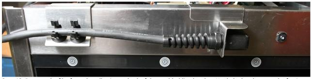
**Step 13**: Remove the film from the adhesive on back of the cord-holding bracket. Hook the bracket over the fascia (**DO NOT** place over circuit breaker.) and hold firmly to the cabinet for 10 seconds. Attach cord to bracket.
