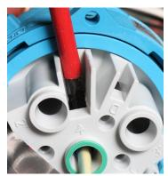
**Step 7:** Set screws secure the leads to the plug. Use a 3/16" precision-tip screwdriver to loosen set screws.
