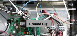
**Step 5:** Remove the power cord, which is attached with spade terminals to the relay, circuit breaker and with a ring terminal on the ground lug.
